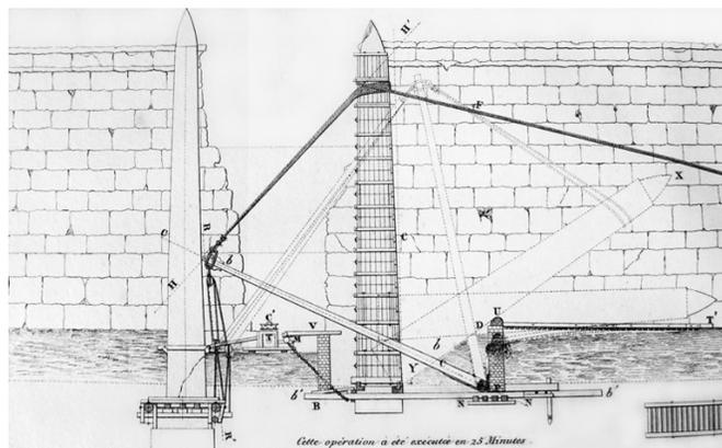
Figure 2: The apparatus designed by Lebas for lowering the obelisk
