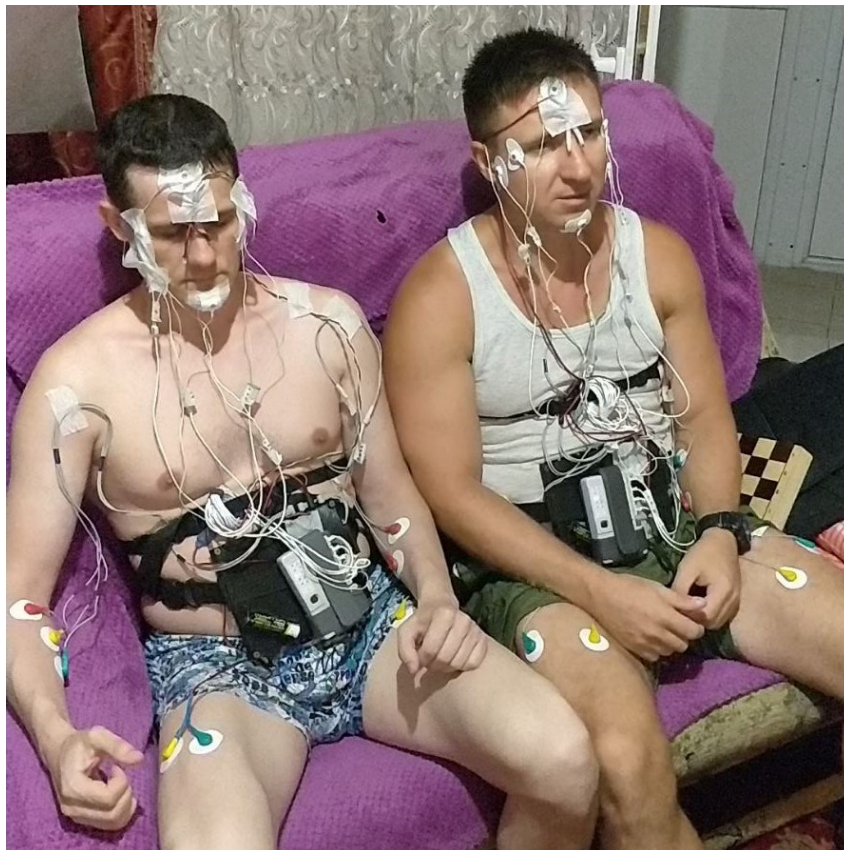
Image 2. Positions of Encephalan-EEGR-19/26 (white), custom-made EMG device (black), EEG/EOG/EMG sensors, diodes, and vibration motors.
