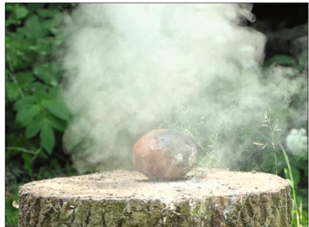
Fig. 13 The effect of pouring half a glass of water over a recent clay ball with a temperature of about 200°C. – (Photo E. Mols).
