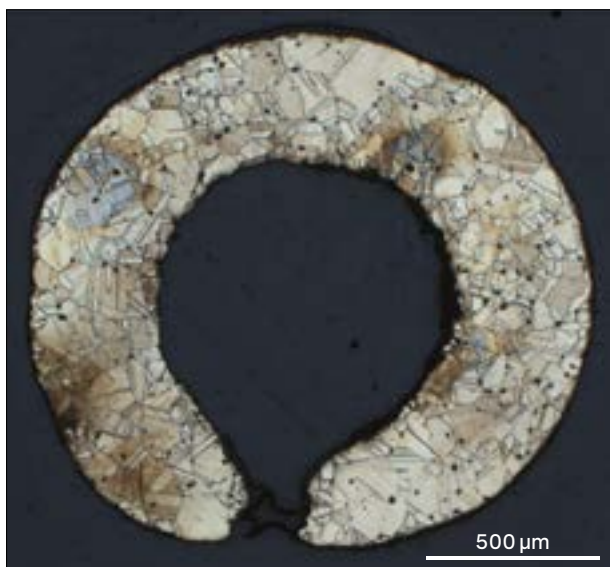
Fig. 7 Photograph and metallographic image of lace chapes (inv. no. A452210). – (Photos M. Kmošek).
