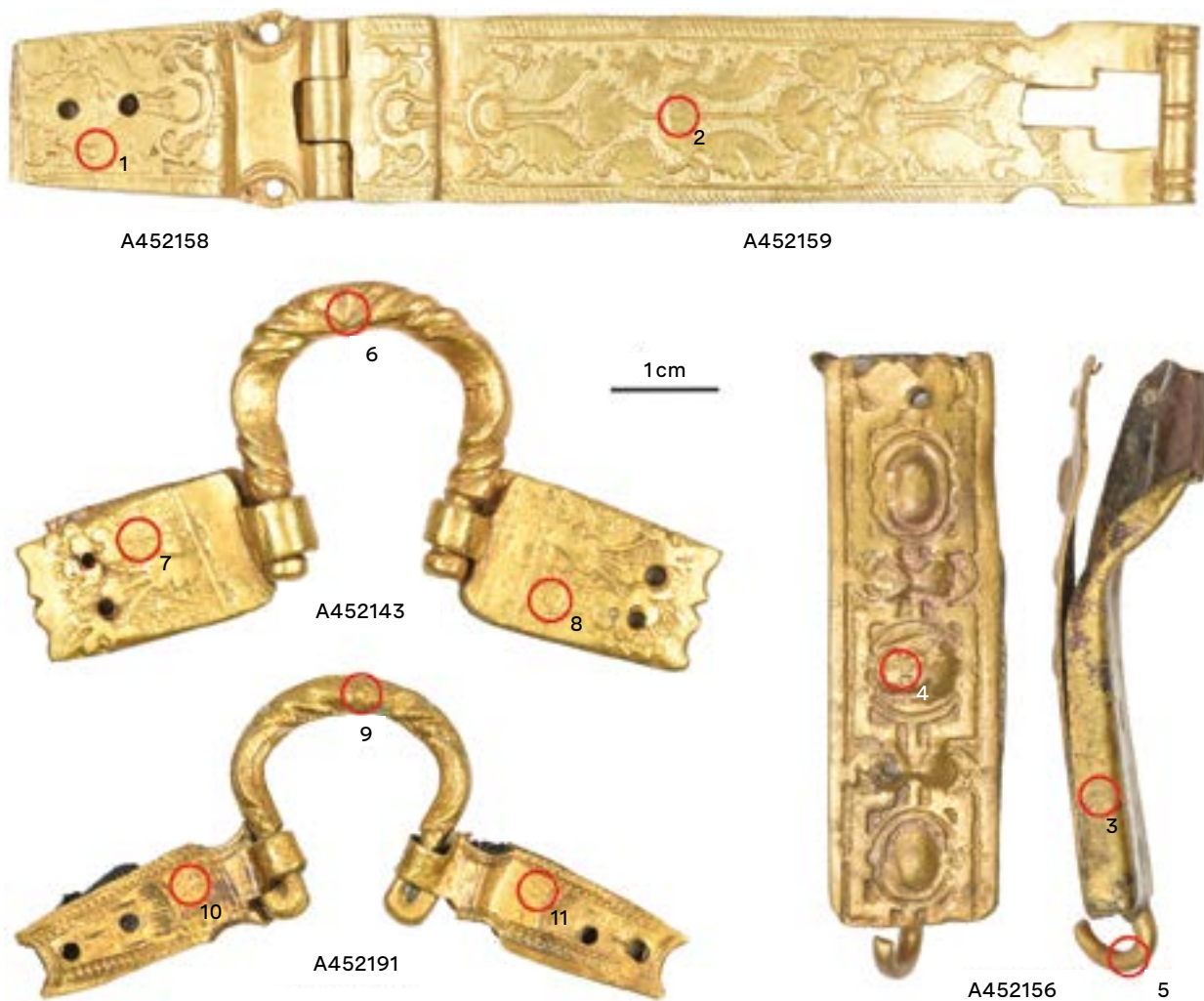
Fig. 11 Composite segmented girdles with positions of the pXRF analysis of their different parts. – (Photos M. Kmošek).
