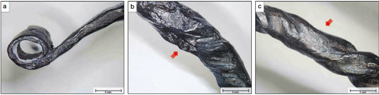
Fig. 19 Photomicrographs of the iron necklace MOP-14. The arrows indicate (b) iron delamination resulted from insufficient treatment of the metal in the post-smelting stages and (c) an area with a change of the twisting direction of the iron rod.
