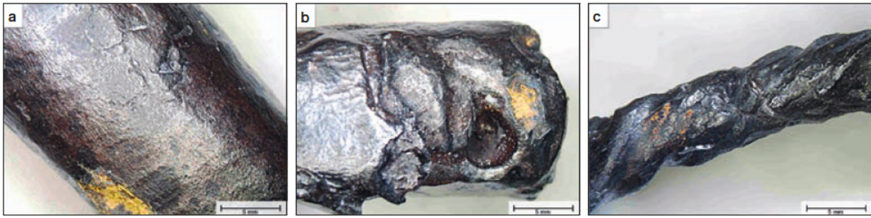
Fig. 23 Photomicrographs of iron metalwork from the Grabionna hoard showing the presence of yellow corrosion products that are associated with the weeping iron condition: a chisel MOP-7. – b socketed axe MOP-12. – c necklace MOP-14.
