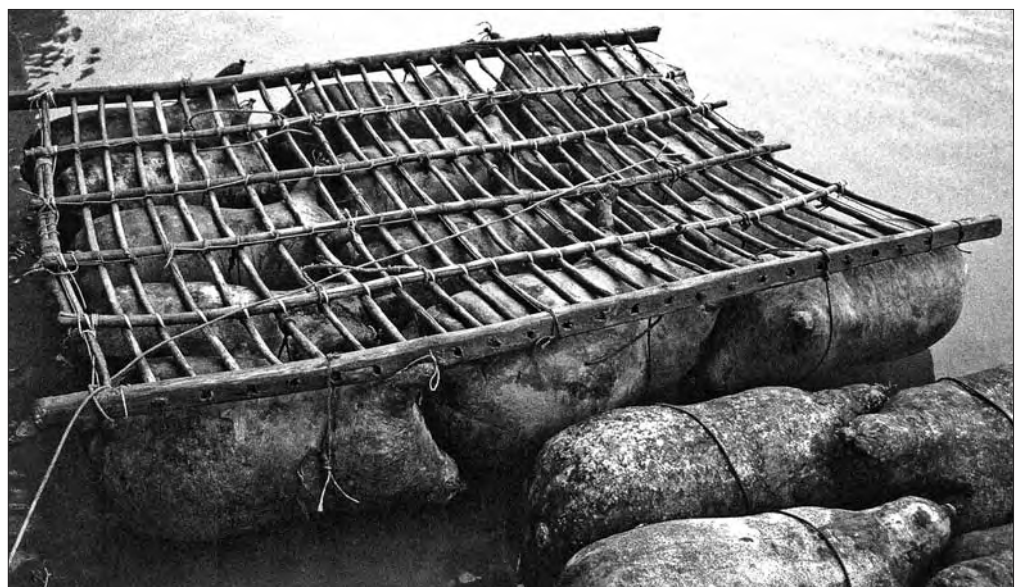
Fig. 1 Raft buoyed by inflated skins on the Huang He river in 2002. – (After Bockius 2007, 13 fig. 6).
