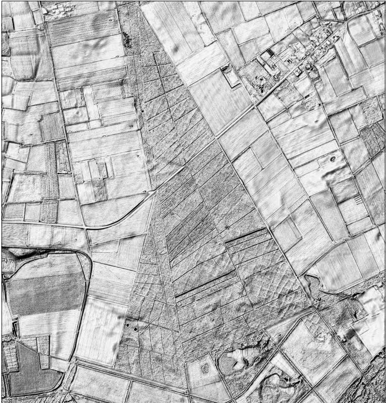
Fig. 5 Sky view factor visualization of the Muisvenner-Ophovenerheide complex (prov. Limburg/B). – (Illustration DTMF, © Agentschap Geografische Informatie Vlaanderen).
