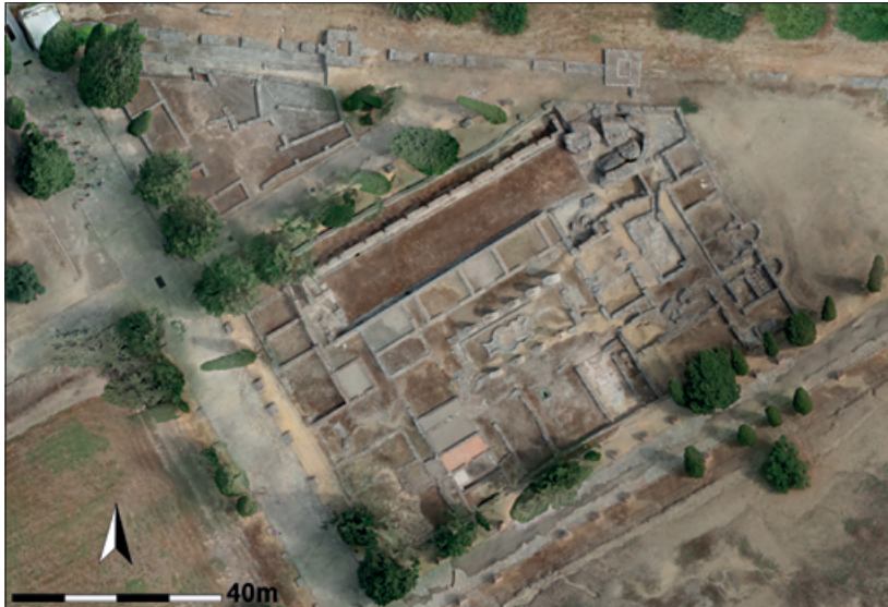
Fig. 5 Italica (Santiponce). Orthophoto of the Casa de la Exedra and the section of the city wall just north of the mansion, taken using an UAV. Spatial resolution is 5.3 cm per pixel. – (After Salzmann 2016, fig. 2).
