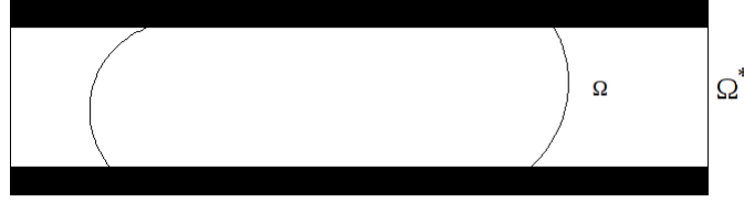
Figure 2.1: The basic configuration of an electrowetting on dielectric device [Cho et al., 2001, 2003]. The solid black region depicts the dielectric plates and the white region denotes a droplet of one fluid (say water), which is surrounded by another (air). We will denote by \Omega the fluid domain and by \Omega^* the region occupied by the fluids and the plates. The boundary between the fluid and the plates is denoted by \Gamma and \partial^*\Omega = \partial\Omega^* \setminus \Gamma .
