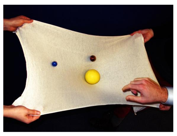
The more concentrated the central mass (i.e., the heavier the large ball), the more curved the bandage will be. This increases the depth of the 'gravitational well' from which the marble will not be able to escape.
