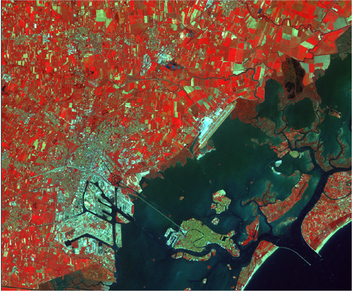
Figure 16: False colour image produced by combining the green, red and infrared bands.
