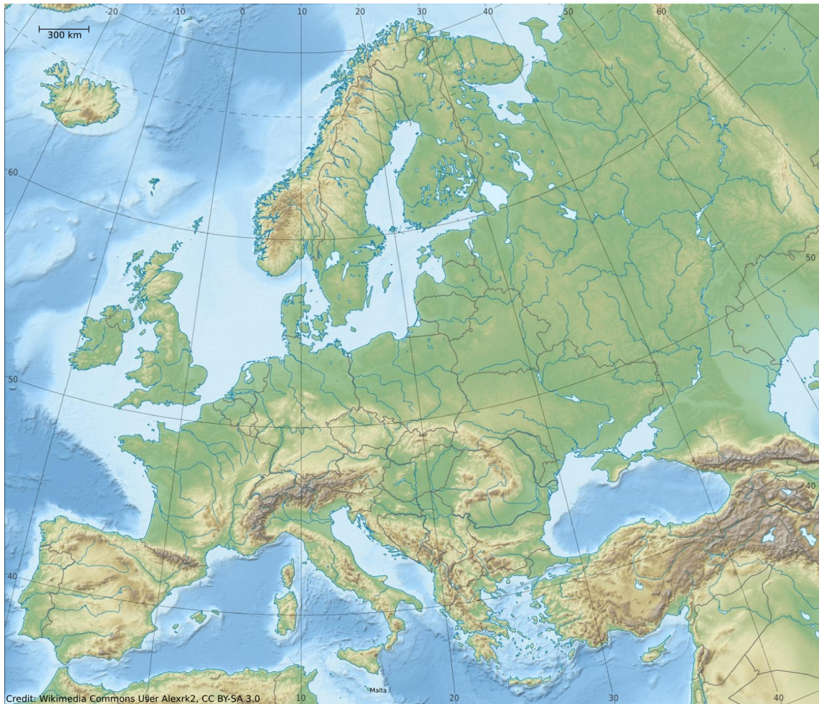
Figure 7: Topographical map of Europe displayed in Lambert azimuthal equal-area projection. This assures a constant scale throughout the entire map. The country borders are indicated with grey lines (Alexrk2, https://commons.wikimedia.org/wiki/File:Europe_relief_laer_location_map.jpg , 'Europe relief laer location map', https://creativecommons.org/licenses/by-sa/3.0/legalcode ).
