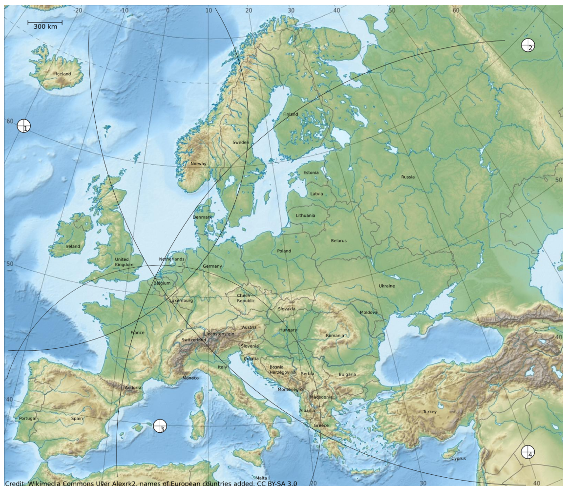
Figure 9: Topographical map of Europe displayed in Lambert azimuthal equal-area projection. The arcs represent the distances that the signals have travelled from the four satellites in the times specified in the table of Worksheet 2 (for credits see Figure 7).
