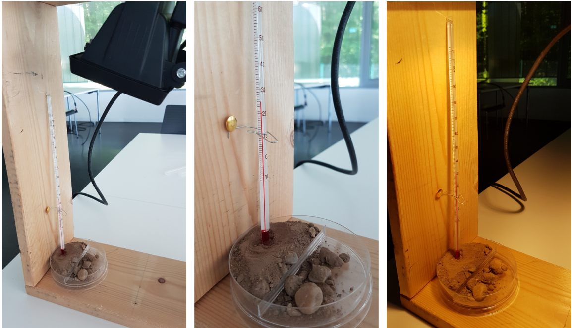
Figure 8: The set-up of the second experiment is the same as for the one with water, but this time the petri dish is filled with dirt, sand, or soil (own work).
