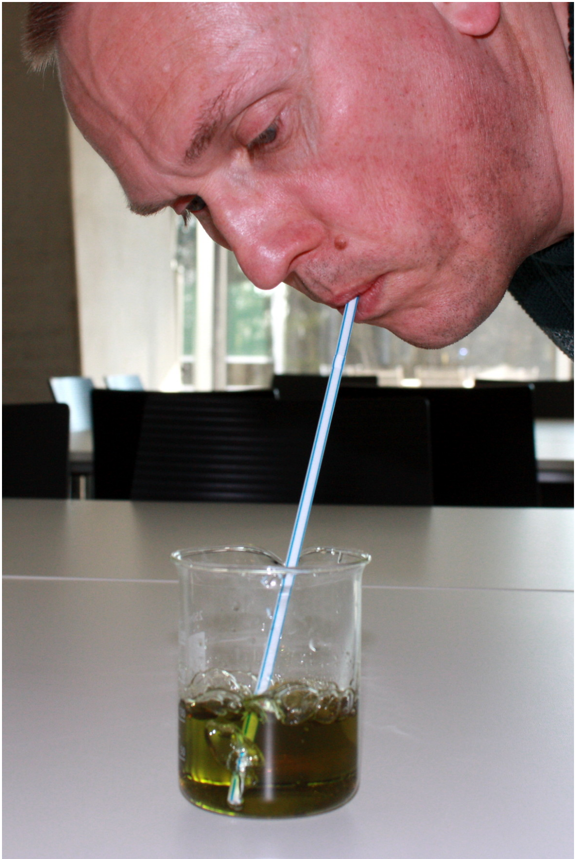
Figure 12: Blowing air into the liquid introduces carbon dioxide, which slowly changes the pH value.
