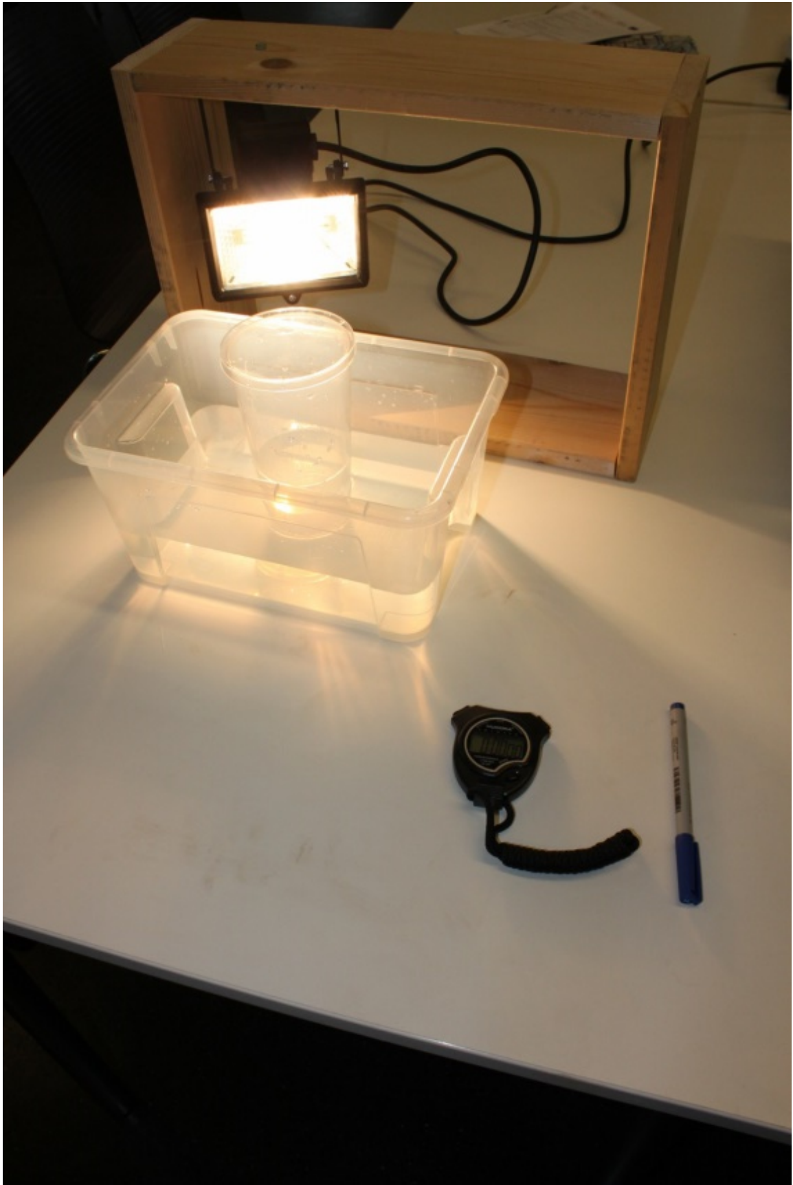
Figure 7: Experimental set-up. A plastic cup filled with water is used as a platform that carries the ice (own work).
