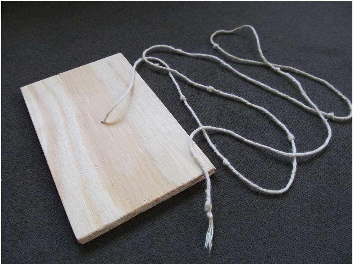
Figure 7: A simple wooden kamal. It consists of a surveying board and a cord with a line of knots (Credit: Bordwall https://commons.wikimedia.org/wiki/File:Simple_Wooden_Kamal_(Navigation).jpg , 'Simple Wooden Kamal (Navigation)', https://creativecommons.org/licenses/by-sa/3.0/legalcode ).
