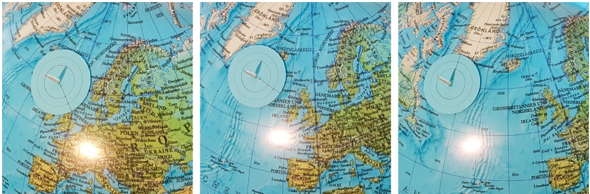
Figure 21: Functionality of the shadow board when travelling west along a latitude. When measured at local noon, the orientation and the length of the shadow remain the same (own work, not presented to the students).
