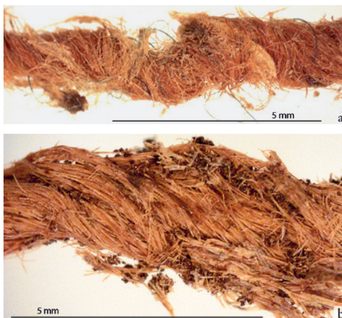
Fig. 131. Optical microscopy images: a. red warp yarns from the upper lining C33208, LH 1969 (1131/21) with several spun blue fibres; b. yarn from blanket textile 2.2 (grave 2), LH 1995 (11132/39) with blue particles or aggregates (photo: I. Vanden Berghe).
