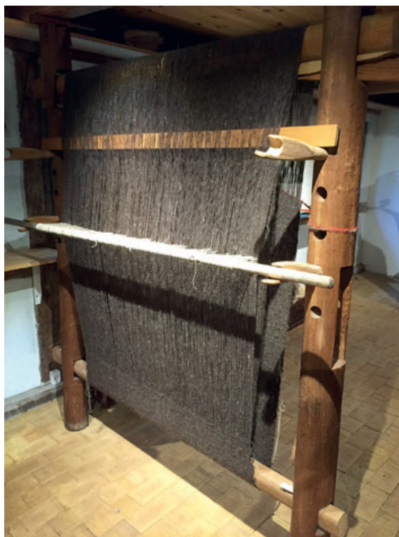
Fig. 21. Reconstruction of a two-beam loom with a tubular warp at Sagnlandet Lejre 2018. The locking cord is the read cord visible in the back layer (photo: I. Demant).
