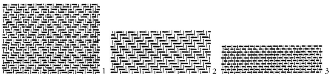
Fig. 18. Schematic overview of the different weaves used at Lønne Hede. 1. twill; 2. 2/1 twill; 3. tabby (after ANDERSSON 2003 fig. 6).
