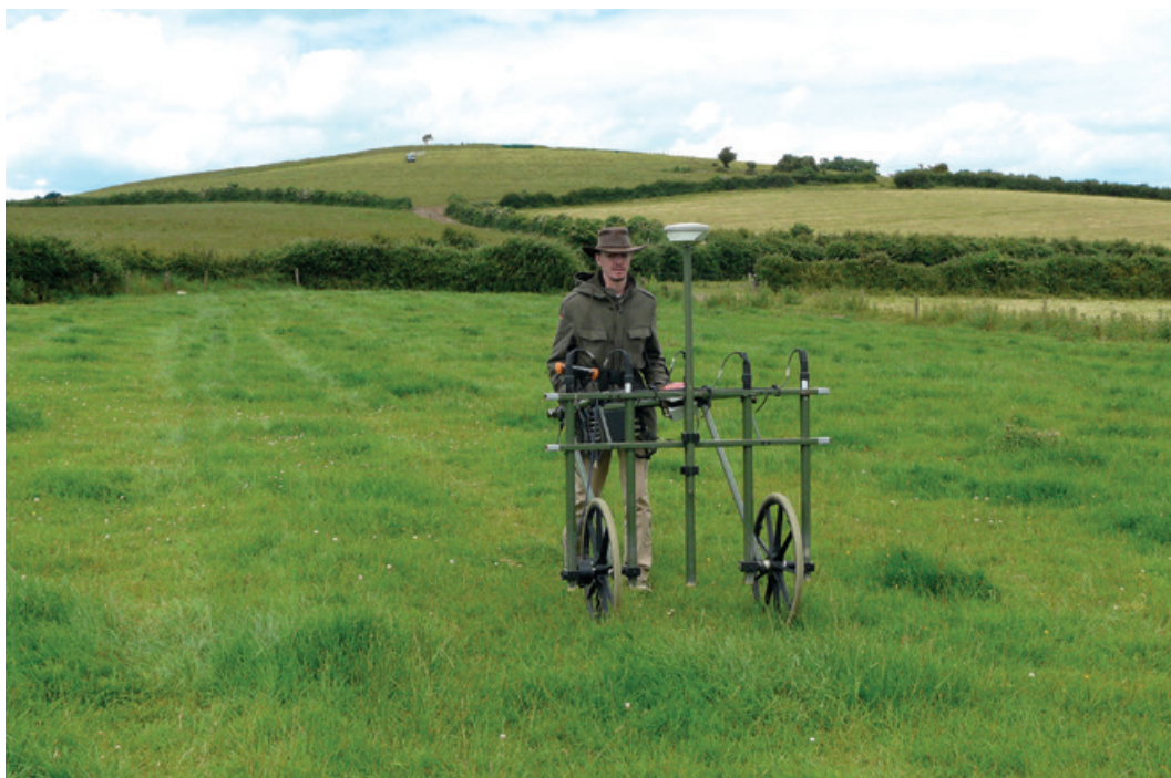
Fig. 3. In the foreground Swen Heinermann and the 5-channel magnetometer, in the background the Freestone Hill hillfort (photo: H.-U. Voß, RGK).
