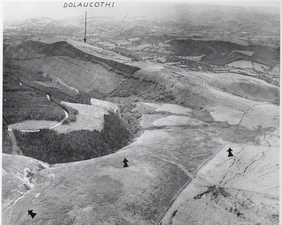
4 The line of the Annell aqueducts (arrowed) at the head of the Annell valley as seen from the east. The line of the Cothi aqueduct runs along the far side of the middle ridge to the minehead.
