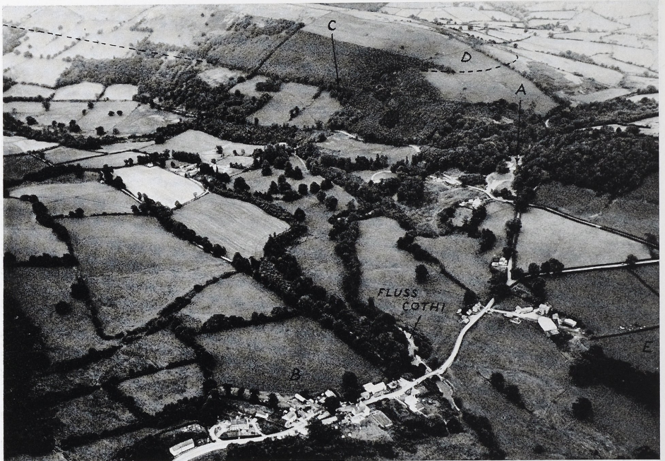
2 Aerial photograph of the main mining area, Dolaucothi, from the west. A = the main opencast at the foot of Allt Cwmhenog ridge; B = site of Roman settlement beneath the present village of Pumsaint; C = level of Cothi aqueduct; D = level of Anell aqueduct; E = site of Roman baths.
