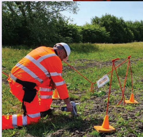
A geochemical sample being taken in the field using the portable XRF machine (© HS2 Ltd)
