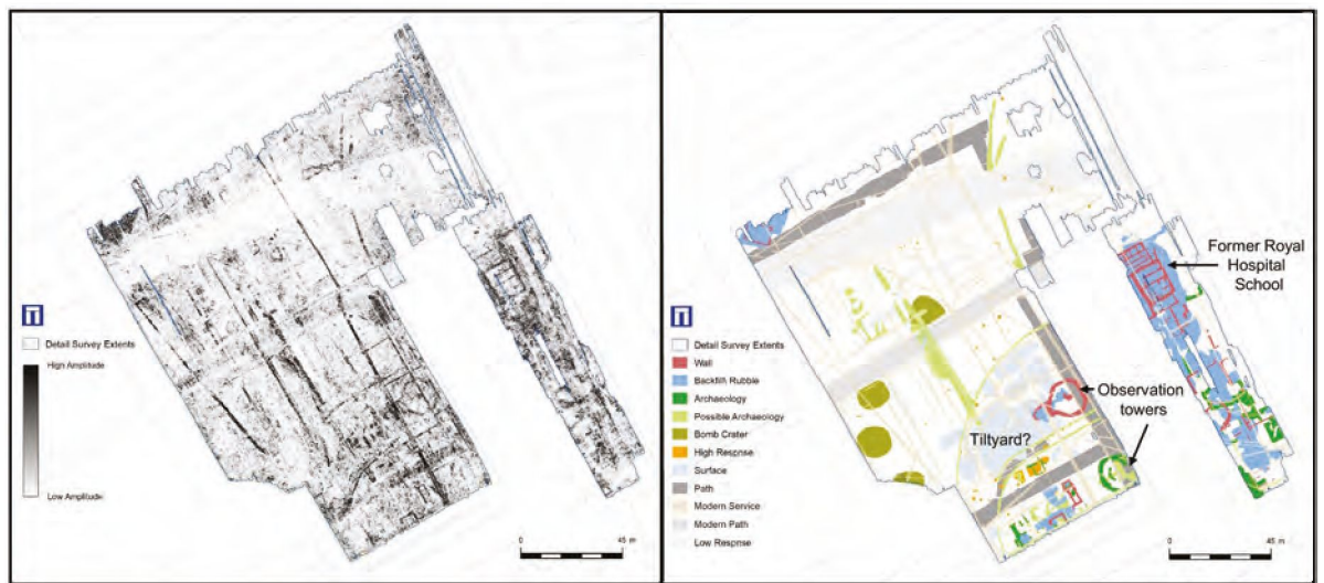
Greyscale plot and interpretation of multi-channel GPR survey from Queen Anne's house in Greenwich, illustrating the location of the observation towers of King Henry's tiltyard. Digital data reproduced from Ordnance Survey data. Credit: Crown Copyright (2020) All rights reserved. Reference Number: 100022432.
