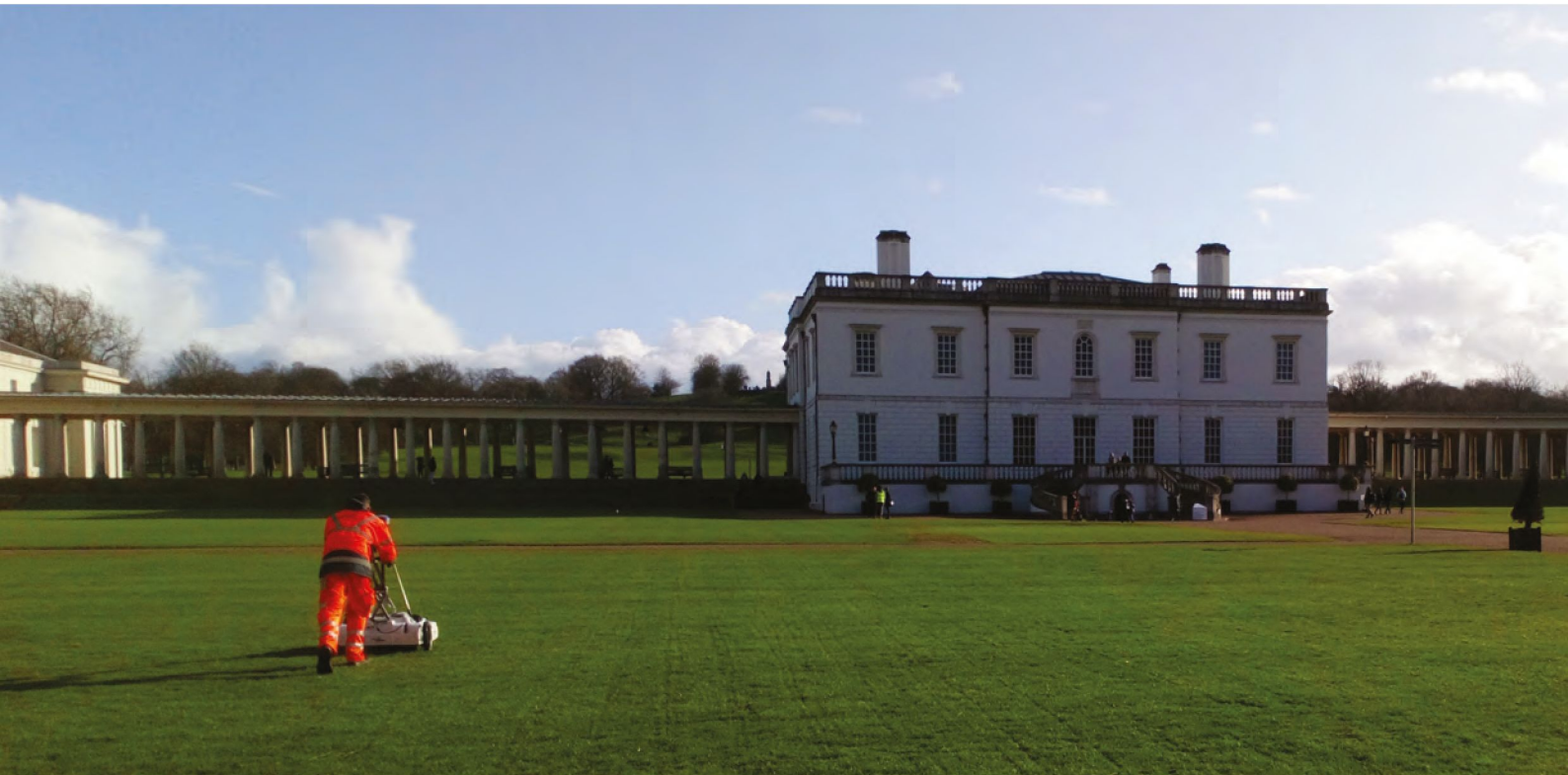
Multi-channel GPR survey in progress at Queen Anne's house in Greenwich, London (NHLE 1002060). The survey was undertaken using an Impulse Radar Raptor array, which contains eight transmitter and receiver antennae spaced 8cm apart, with a central frequency of 450MHz. Credit: Wessex Archaeology
