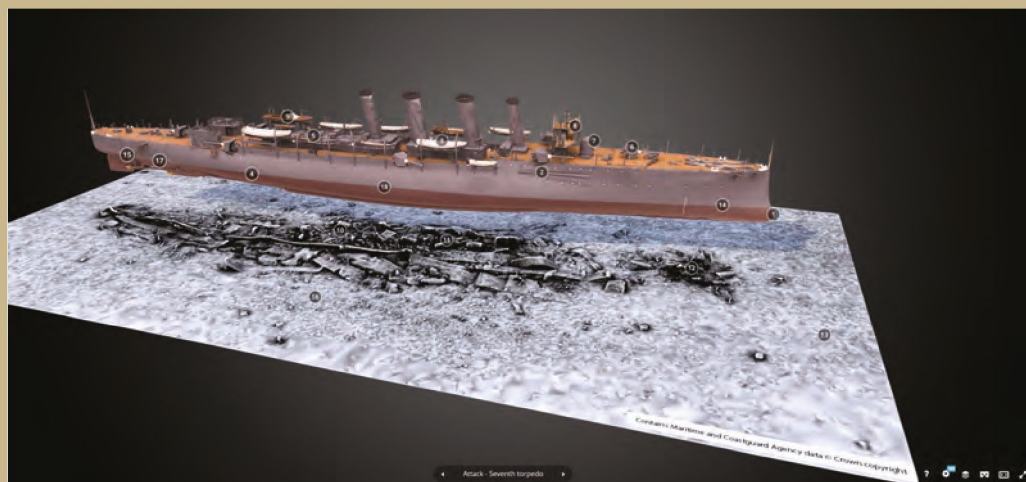
3D model of the 1911 builders' model of HMS Falmouth positioned over MBES data showing the wreck today. Features can be identified by clicking on the numbered information points. Full model available at https://historicengland.org.uk/research/current/discover-and-understand/military/the-first-world-war/first-world-war-home-front/what-we-already-know/sea/hms-falmouth/ . Credit: Fjordr Ltd/Historic England
