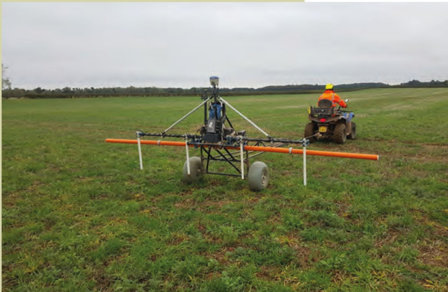
Simultaneous collection of magnetic (vertical white sensors) and EM (horizontal orange sensor) data on a larger scale. Credit: Magnitude Surveys Ltd
