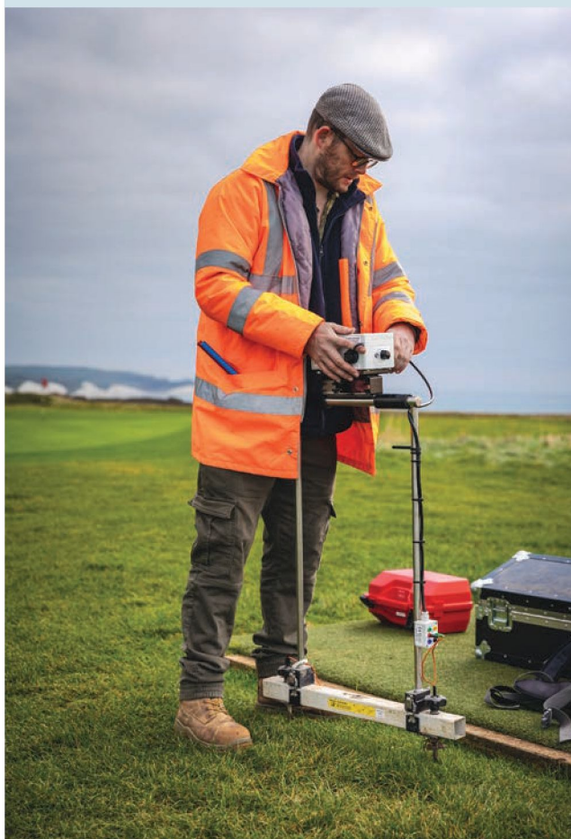
Ed Blinkhorn setting up resistivity survey. Credit: Chip Creative
