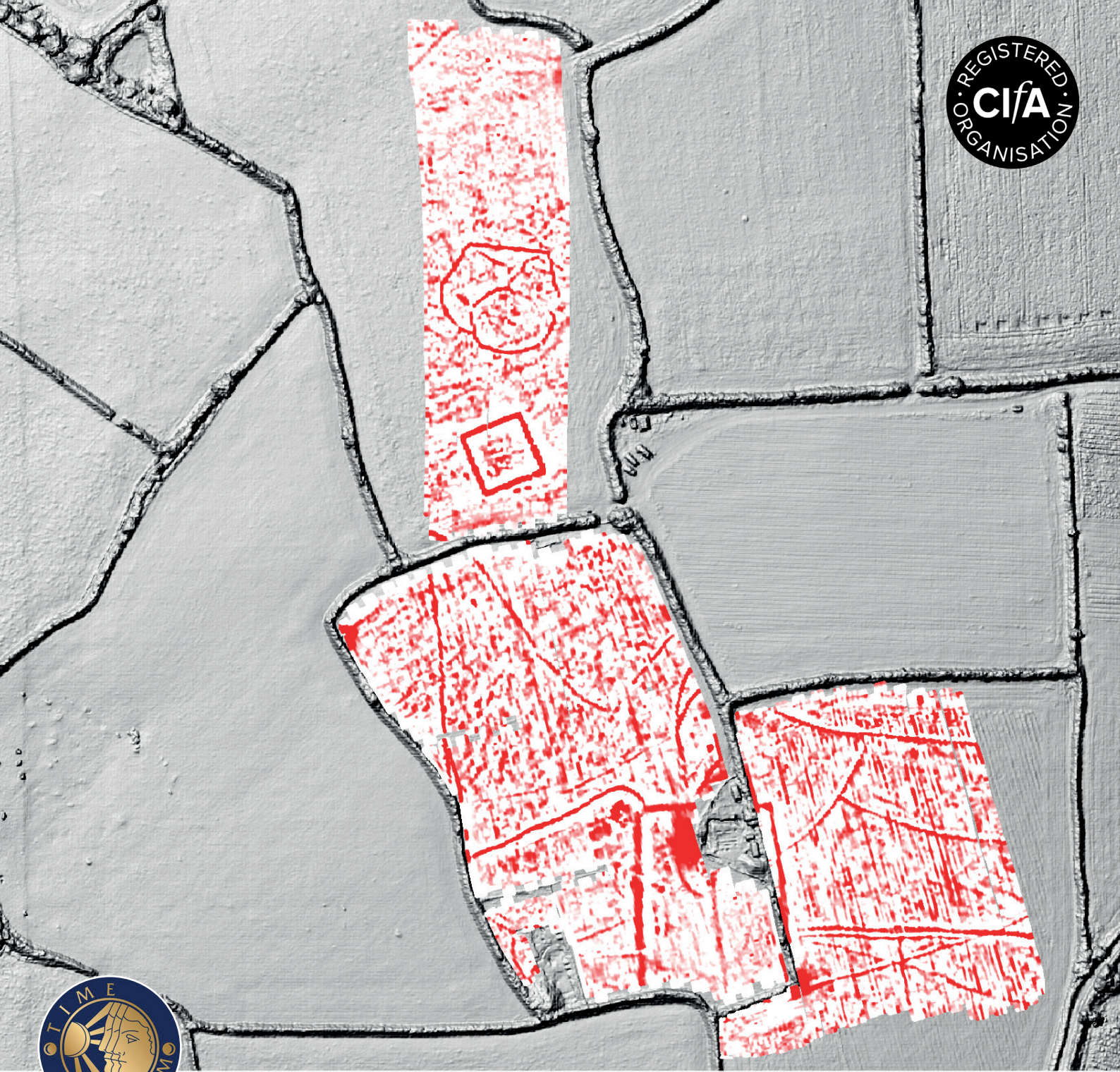
Magnetic data superimposed over UAS Digital Elevation Model for Time Team 2022
