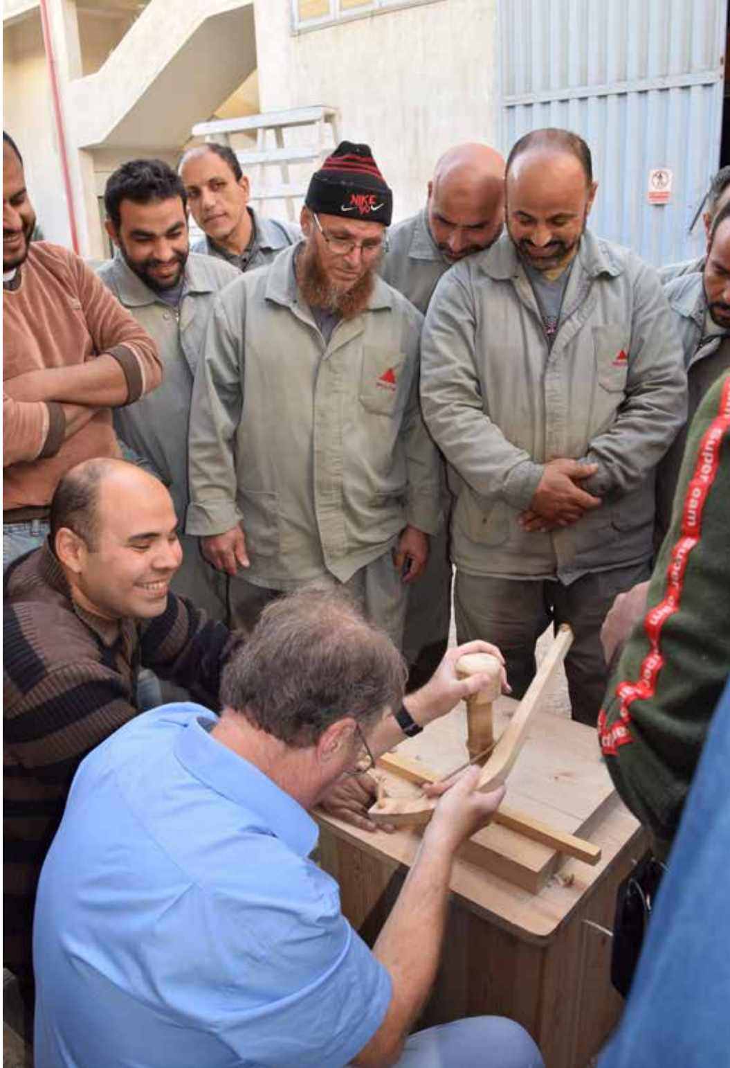
Fig. 6: Dr Geoffrey Killen and Dr Nour Mohamed Badr demonstrating the bow drill with carpenters at the Pinocchio furniture factory in Damietta. (Image © Fitzwilliam Museum Cambridge.)
