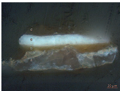
16 Cross section of the white paint layer from the bottom of the casket (ground layer is missing): corroded tin-foil (a), gold-coloured lacquer (b), white paint (c), varnish (d)
