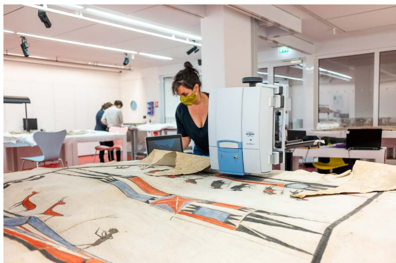
2 Installing the Fourier-transform infrared spectroscopy unit, to analyze the physico-chemical constituents of the painted hide
