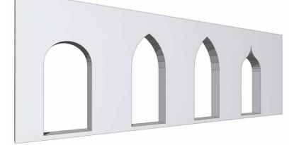
Figure 7: Arched opening with parametrically controlled dimensions and arch type.
