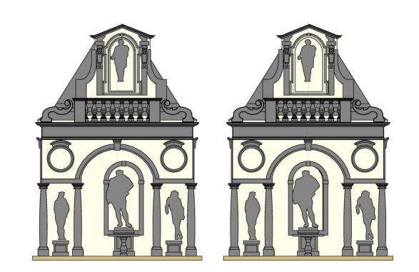
Figure 3: Schematic rendering of two survey drawings of the garden pavilion of the Rubens' House, showing slight differences in the placing of the statues.
