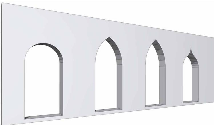
Figure 7: Arched opening with parametrically controlled dimensions and arch type.
