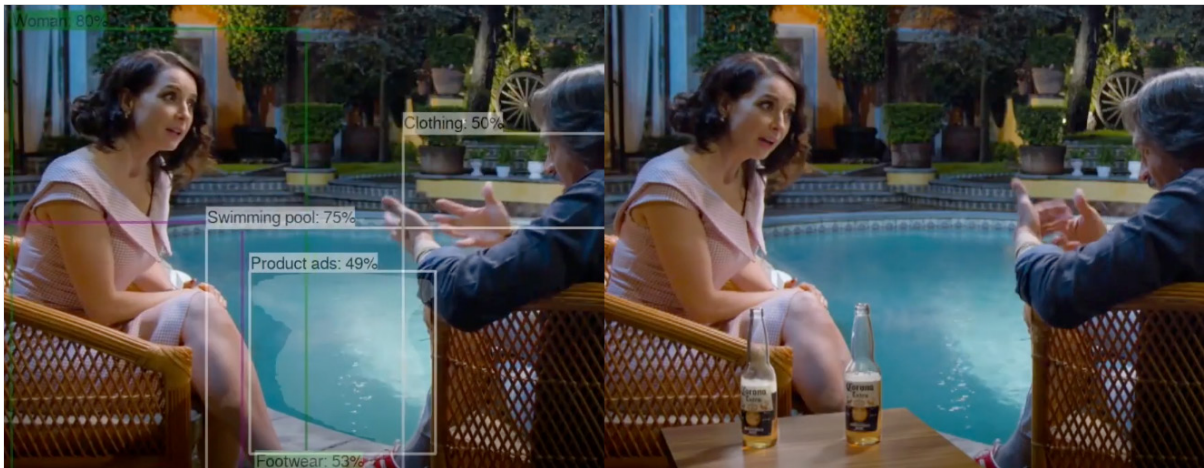
Figure 6. Mirriad Inc.; 2019; https://youtu.be/npW00TW0WLE ; Rendering virtual content into a video based on image analysis using artificial neural networks.
