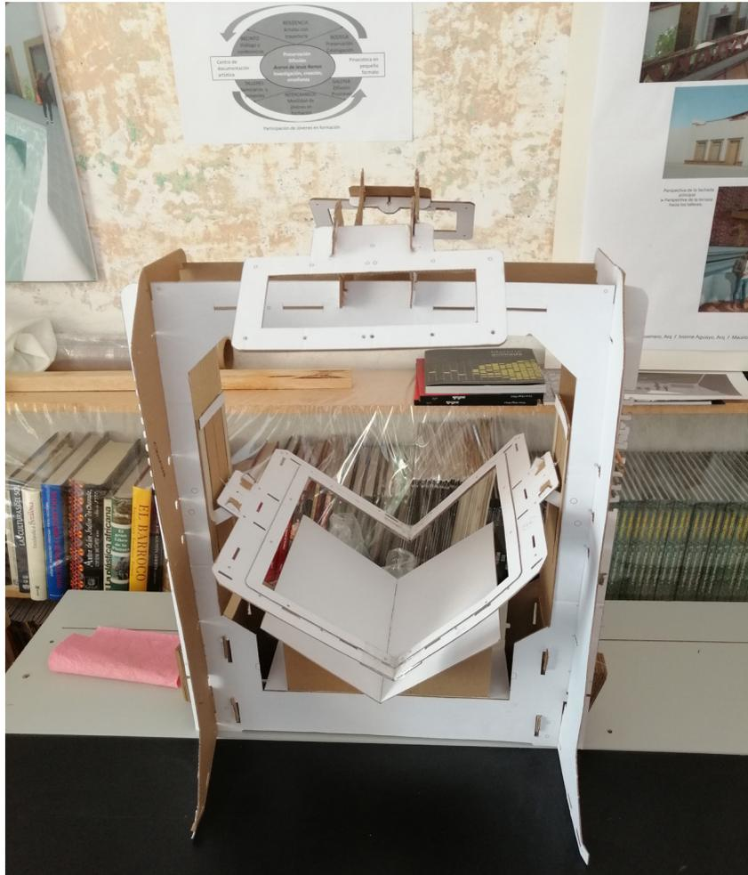
Figure 9. Prototype for one of the scanners used in the documentation center, based on blueprints provided by BiblioHack.
