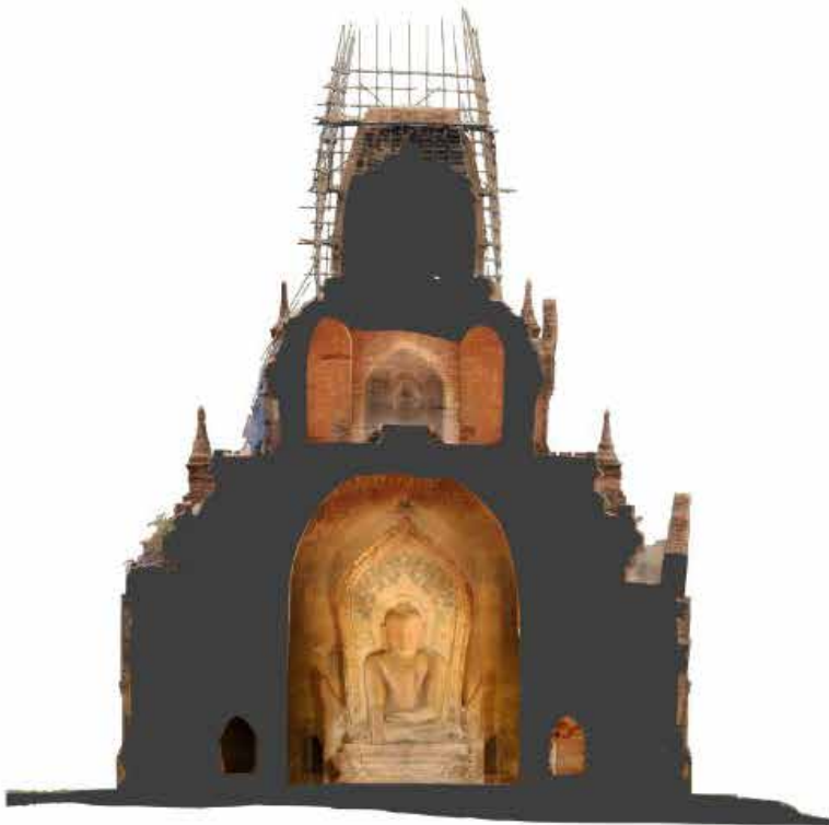
Figure 5: Exterior elevations (top) and clipped interior sections (bottom) of temples at Bagan. Center, (bottom and top): Eim Ya Kyaung temple. Left and Right (bottom and top): Khemingazedi temple.
