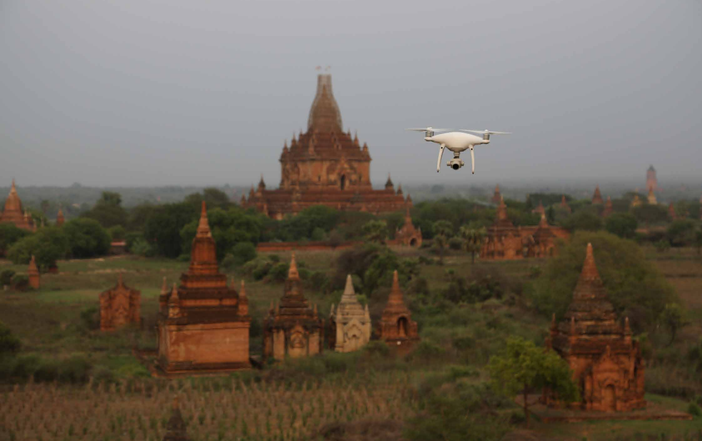
Figure 3: Drone at Bagan, Myanmar: aerial photographs captured by a remote-controlled drone provide images of surfaces, such as rooftops, that are inaccessible to the scanner; digital models of these features can be generated from the images and combined with laser scans using photogrammetry software. Photo by Kieran Kesner for CyArk.
