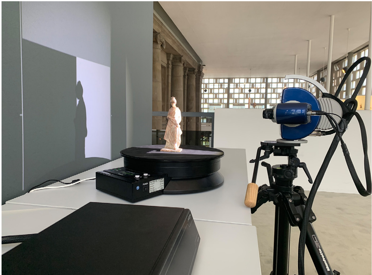
Figure 3. Acquisition of 3D-models of terracotta figurines at the Museum August Kestner, Hanover. © JfDH.
