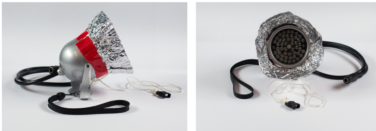
Figure 5: Near infrared BW® 48 LED Illuminator (30° beam spread) employed for Test 2 with customised light throw attached.
