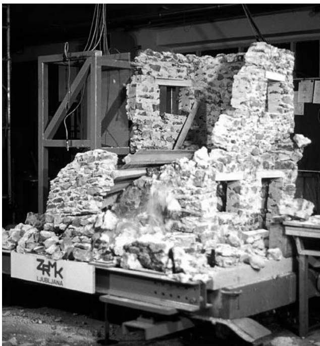
Fig. 8a and 8b Results of a shaking table test using a model of a rural stone house with wooden floors; (a) without steel ties, (b) with steel ties
