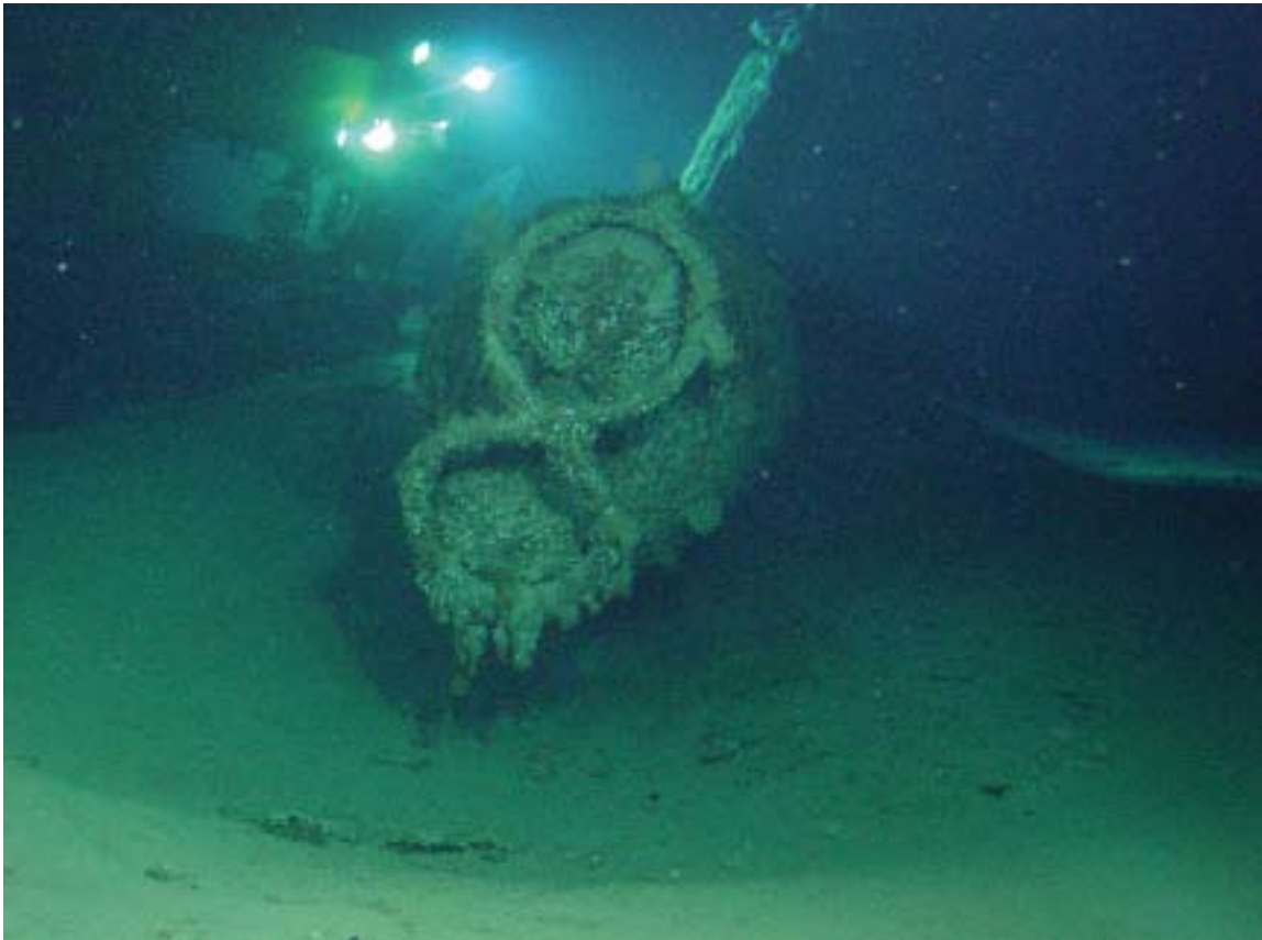
Figure 2: Torpedoes at bow and current scour beneath the forward section (image HURL 2002)
