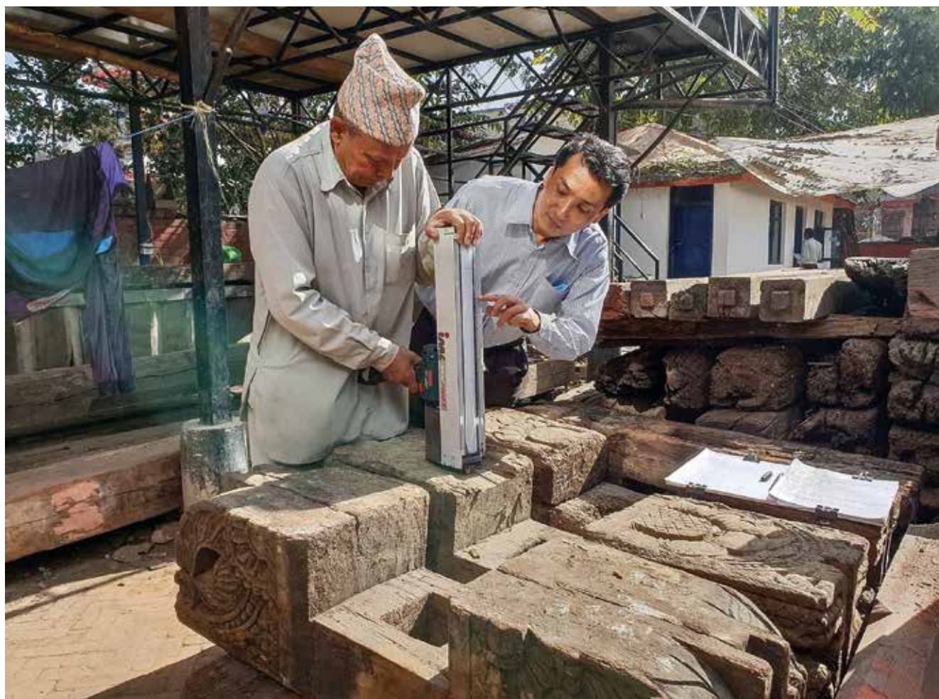
Fig. 4b: Traditional artisan and head carpenter Laxmi Bhakta Rajchal trying out a resistograph, assisted by Project Manager and ICOMOS Nepal Secretary Manindra Shrestha (© ICOMOS Nepal/Anie Joshi)
