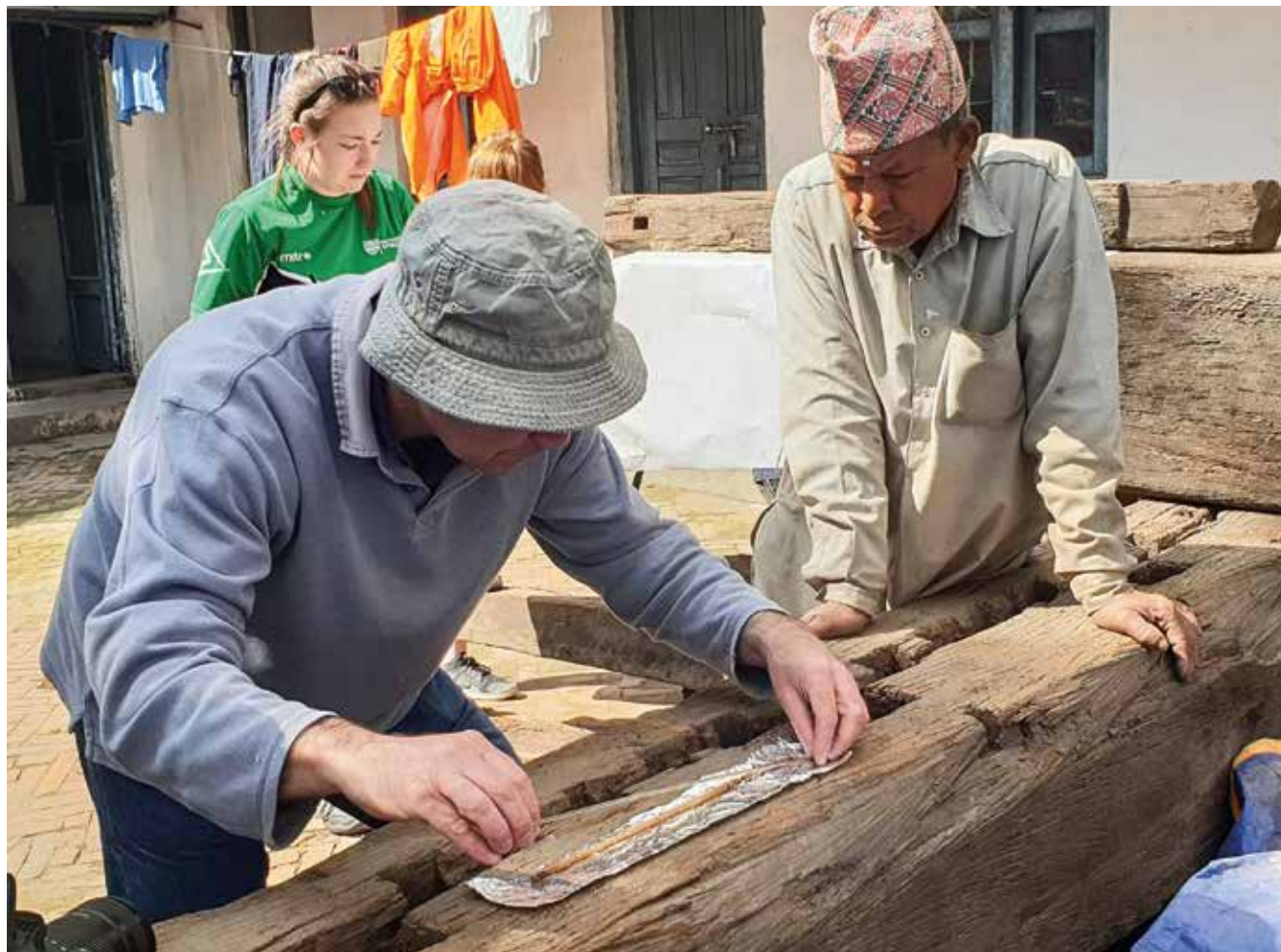
Fig. 4a: Professor Simpson from Sterling University in Scotland taking a wood sample for testing and dating while the traditional artisan and head carpenter Laxmi Bhakta Rajchal looks on (© ICOMOS Nepal/Anie Joshi)
