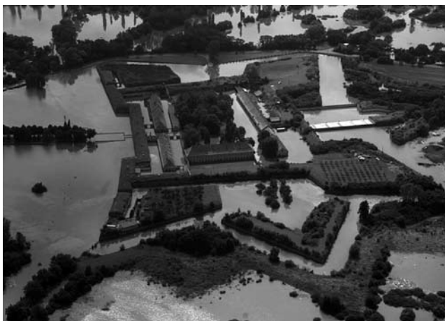
Fig. 7 Terezín, fortress. The original fortifications are based on Baroque fortification systems of the 17th century. During the August 2002 floods, Terezín and surroundings were flooded up to a height of 3 meters. The historically valuable underground protection system of the fortress was also badly damaged.
