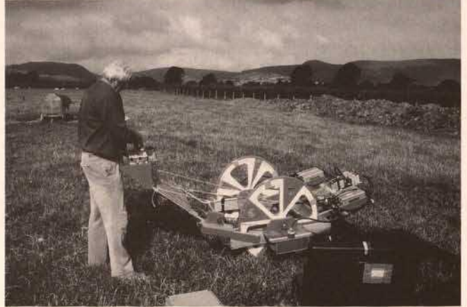
Fig. 1. "Magneto-Scanner" in Hindwell 1998; four caesium magnetometers Scintrex SMARTMAG SM4G-Special with quadro-sensor configuration, two gradiometer consoles-data loggers, power supply (4 batteries 12 V/6 Ah) and automatic distance trigger mounted on a nonmagnetic chariot, total weight about 60 kg), type II/1996
