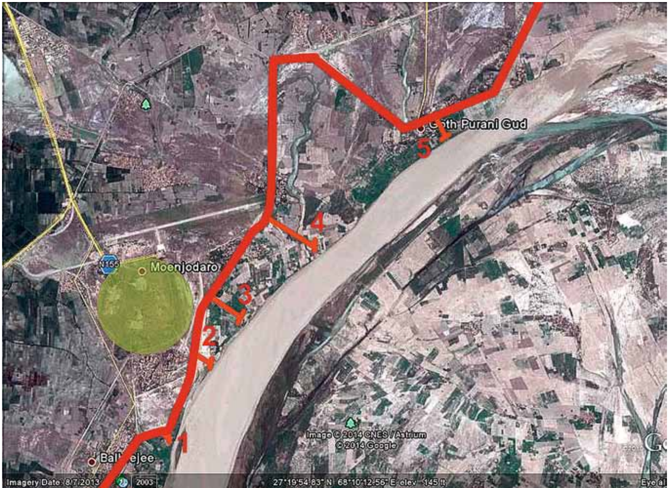
Fig. 11: Mohenjo-Daro, outer bund embankment showing five T spurs which divert flood waters away from the site
