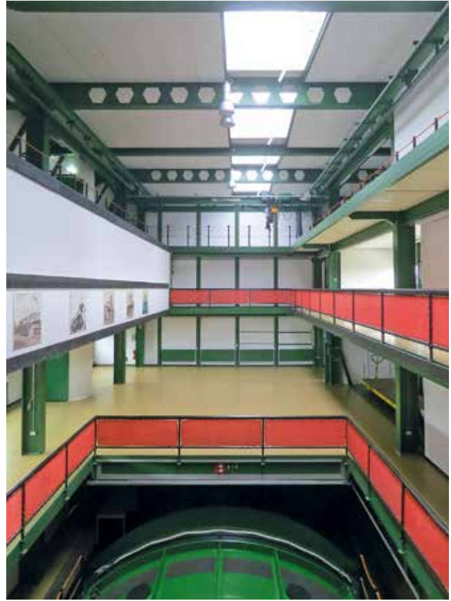
Fig. 8: The decks of the laboratory; the top of the water tube appears on the lower deck, painted green (© adb Ewerien und Obermann)
