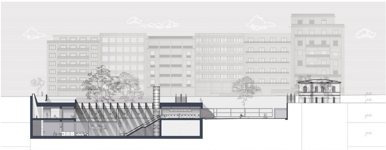
Fig. 9: Section along the entrance level, alternative proposal for the new Evangelismos station. Source: Venetsanaki Charikleia
