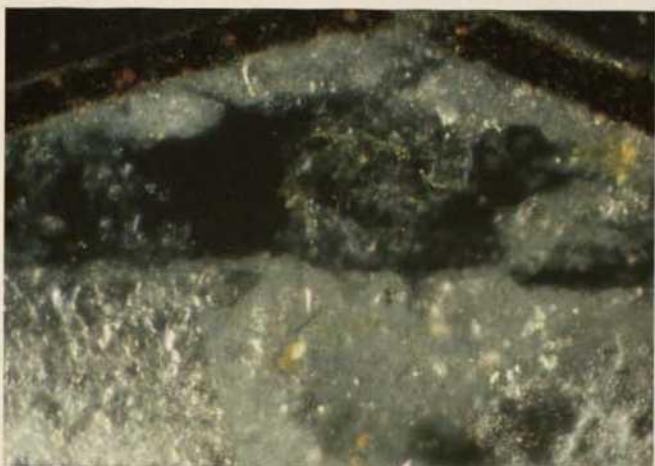
Fig. 5b. Padua, Scrovegni-Chapel: Stratigraphic section observed at transmitted light, crossed nicols, ob. 10x. Gypsum crystallization is visible under the pictorial layer.
