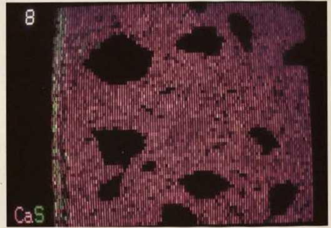
Fig. 4. Padua, Scrovegni-Chapel: X-Ray map at SEM + EDS of calcium (pink) and sulphur (green), 80x.
