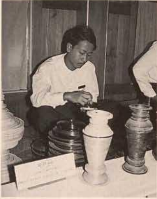
Fig. 9. First stage of lacquer coating
