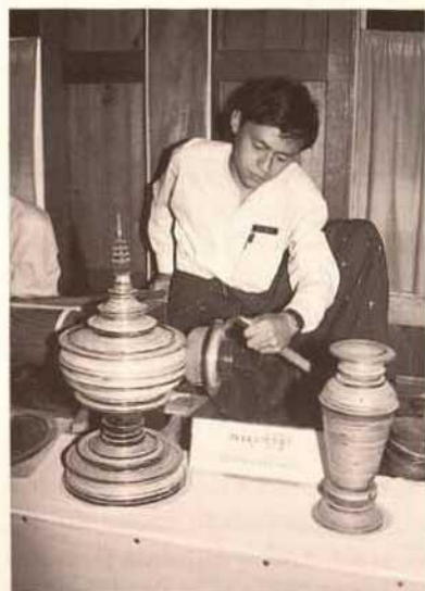
Fig. 6. Finishing the surface of bamboo bodies
