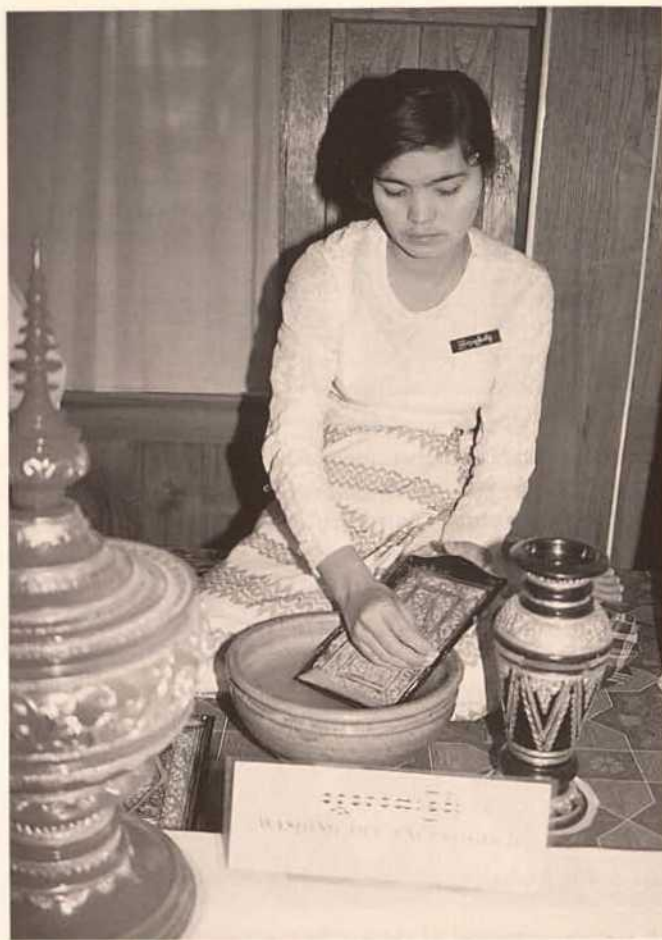
Fig. 15. Washing away the resin mask with clean water. After the removal of the mask the ground colour (black or red) reappears forming a contrast to the gilded design
