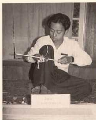
Fig. 2. Bamboo is sliced into narrow pieces and cleaned thoroughly before a body can be formed
