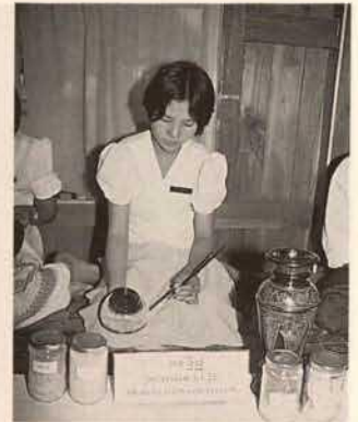
Fig. 10. Last stage of lacquer coating. The lacquer coating is finished when a shining black surface is obtained as shown to the right
