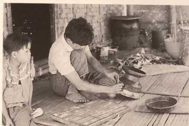
Fig. 19. Gilding of the surface with gold leaves
