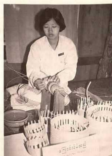
Fig. 8. Sliced bamboo stripes are wound to form a body with the support of a wooden mold
