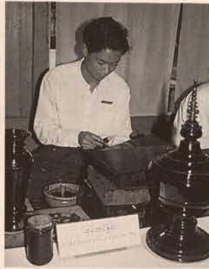
Fig. 10. Last stage of lacquer coating. The lacquer coating is finished when a shining black surface is obtained as shown to the right
