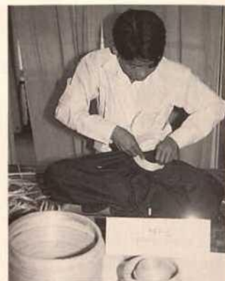
Fig. 2. Bamboo is sliced into narrow pieces and cleaned thoroughly before a body can be formed
