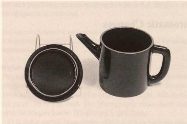
Fig. 1. The interior of the lid of this Japanese sake pot has turned from lustrous black to opaque beige in colour
