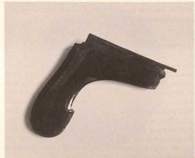
Fig. 5 a–c. Waterlogged wooden bodies of lacquer after treatment with mono-glyoxal and additional agents
