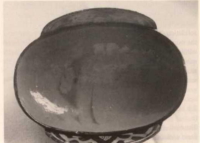
Fig. 5 a–c. Waterlogged wooden bodies of lacquer after treatment with mono-glyoxal and additional agents
