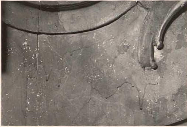
Fig. 3. Side altarpiece of the Catholic Pilgrimage Church at Froschhausen. In the course of earlier restorations it had been partially painted over with a linseed oil-stand-oil lacquer. For this reason the retable shows lacquer runs in several places
