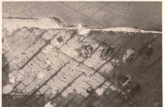
Fig. 2. Cross section of the surface of the veneered high altarpiece at the Church of the Guardian Angels in Straubing under UV-light, 50x magnification. A light-blue fluorescent original lacquer is seen on the wood in the left half of the picture with nearly the original layer thickness. To the contrary, in the right half of the picture it has been reduced to such a degree that it is barely visible on the wood veneer any more. The retouching (yellow fluorescence) lays over both surfaces
