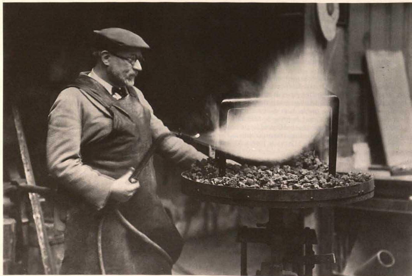
Fig. 14. Jean Dunand demonstrating with a blow torch the fire resistance of a lacquered table, cast with a newly developed material, 1935
